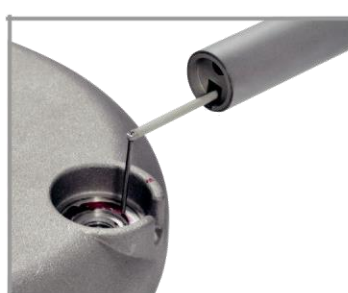
TIME S236 pickup for extra deep groove (20mm)
